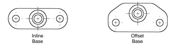
Note: Honda uses two styles of fuel pressure regulator bases. Before proceeding with your installation please compare the fuel pressure regulator on your vehicle and your new AEM adjustable fuel pressure regulator with the above diagrams.
